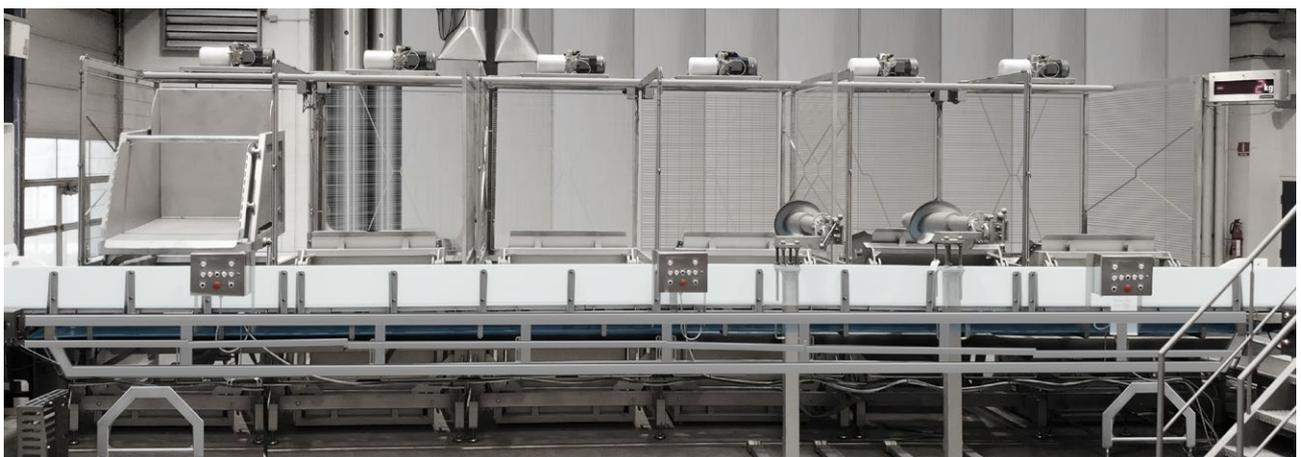
6 (six) unit weighing station, seen from the batching/weighing side. The operator looks at the control panel to the right to check how many kilos he requires of a certain meat raw material. Next, the operator looks at the operator panels in front of each swing loader to see where he has to unload/weigh out the volume of the meat required. The weighing belt is equipped with 4 (four) load cells in order to monitor weights continuously.
