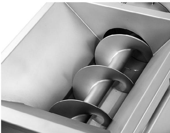
Large diameter infeed screw in horizontal infeed hopper.
