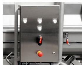
Standard screw conveyor electrical/operator panel.
