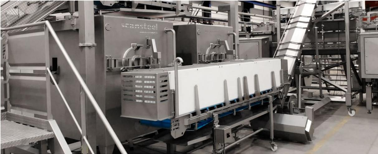
Another typical horizontal belt conveyor solution where 2 (two) grinders are discharging onto the scansteel foodtech® belt conveyor. This solution saves a lot of safety devices and, at the same time, secures easy access to the grinders for cleaning, mounting, and dismantling of the grinders, front view.
