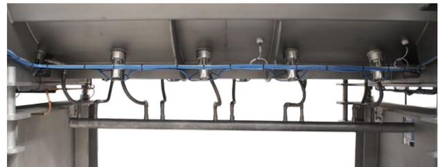
The scansteel foodtech® scanDefrost series has made production logistics much easier, as the meat raw materials to be further processed is taken directly from the freezer without time consuming storage in tempering rooms or other thawing facilities.
