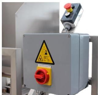
Operator/control panel with emergency stop.
