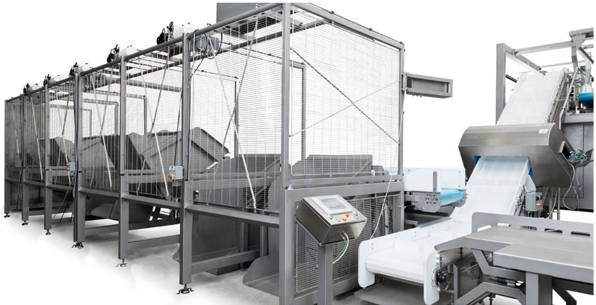
6 (six) unit weighing station, seen from the infed side. Typically, Dolav bins are fed into the swing loaders by a fork lift truck. All is controllable from the operator panel.
