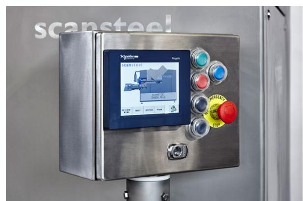
Operator control with easy-to-understand push button operation of start, stop, and emergency. Pre-setting of worm/auger speeds and programming functions with logically designed graphics on the touch panel. Programmes with fixed settings for various products can be keyed in with password protection. The scansteel® scanControl function can be set to optimize the feeding worm/auger speed in relation to the grinding worm/auger, thus reducing grinding capacity flow fluctuations.
