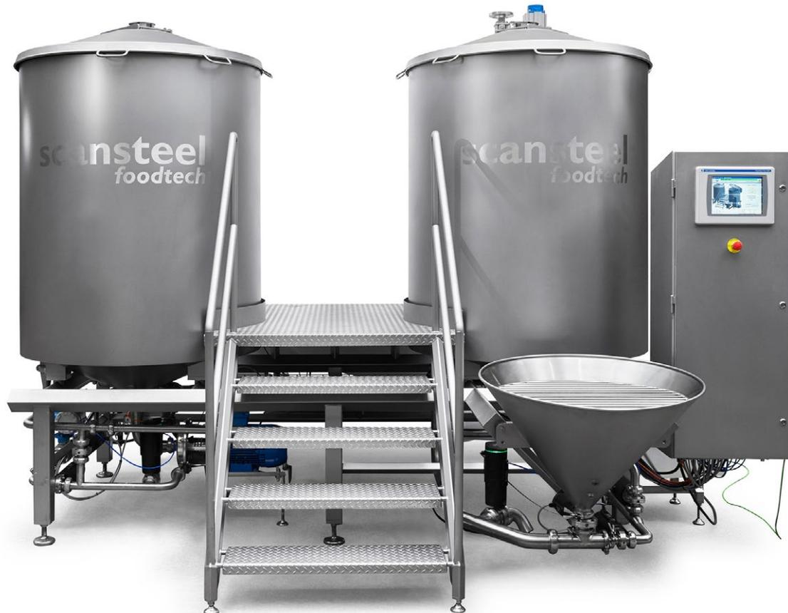
Right hand side: scansteel foodtech® mixing unit with high speed dry ingredients addition Venturi system.
