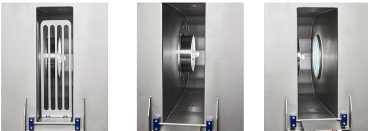
Hygienic zone shown in 3 (three) positions: running position (closed) and cleaning position shown from both angles.
