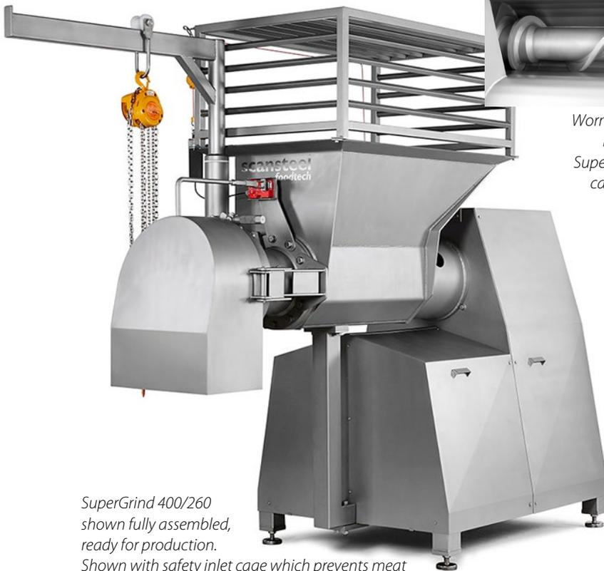
SuperGrind 400/260 shown fully assembled, ready for production. Shown with safety inlet cage which prevents meat raw material, such as frozen blocks, from being ejected during feeding of the grinder.
