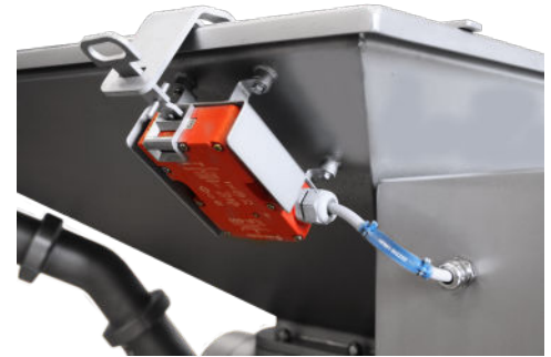
Safety switch for hopper lid.
