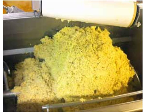
scansteel foodtech manufactures and supplies a range of cheese extruders, model MGX 250/300/400, respectively. The extruder series delivers a high product surface area combined with a high capacity output. Additionally, the extruder series is, as standard, equipped with foreign matter separation.
